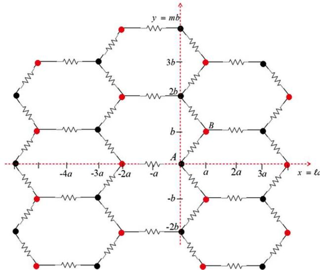
**Fig. 5.** The basal plane (hexagonal lattices) of the hexagonal prism lattice with the two perpendicular coordinates  $\ell a$  and  $m b$ .
