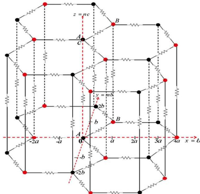
Fig. 4. The resistor network of the three-dimensional hexagonal prism lattice.
