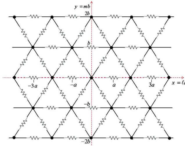
**Fig. 2.** The basal plane (triangular lattices) of the triangular prism lattice with the two perpendicular coordinates  $\ell a$  and  $m b$ .
