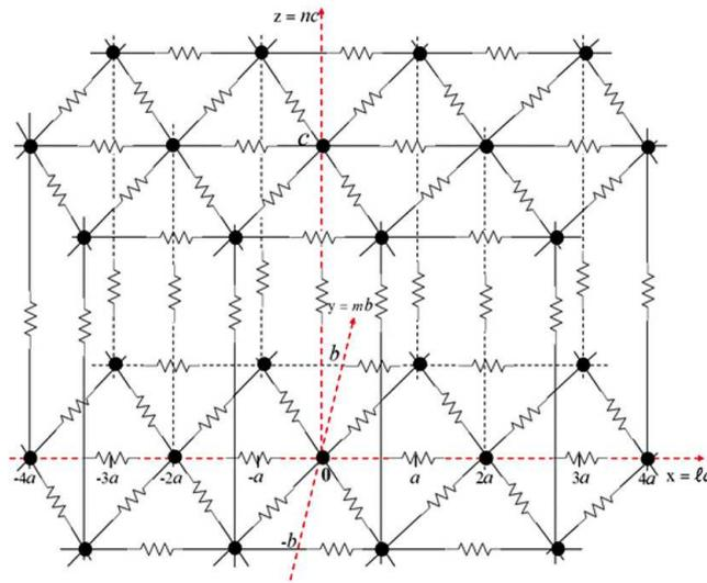
**Fig. 1.** The resistor network of the three-dimensional triangular prism lattice.
